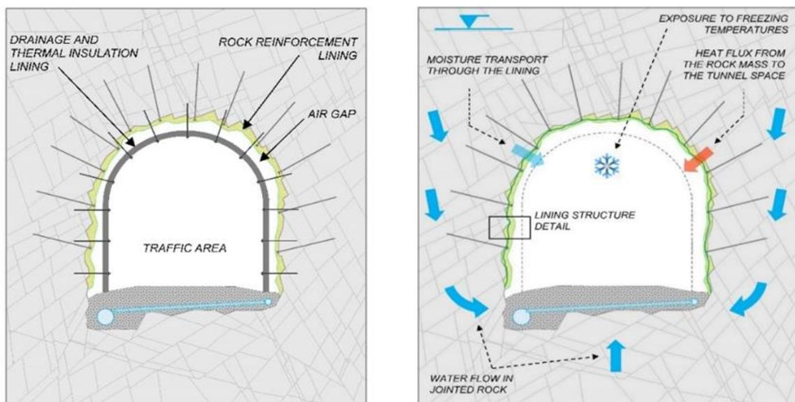
Figure 11: Cross sections of the final inner lining of the Gevingås rail tunnel. Left: Original design with the PE foam sheet drainage system, realized in 2200 m of the tunnel length. Right: the alternative and innovative design with sprayed concrete and spray-applied waterproofing in the final inner lining, realized in 1850 m of the tunnel length. The waterproofing redirects the water flow as shown [7]
