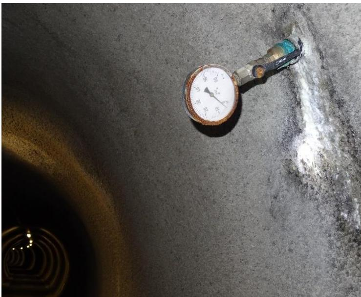
Figure 8: Manometer indicating 4 bar water pressure [Master Builders Solutions]
