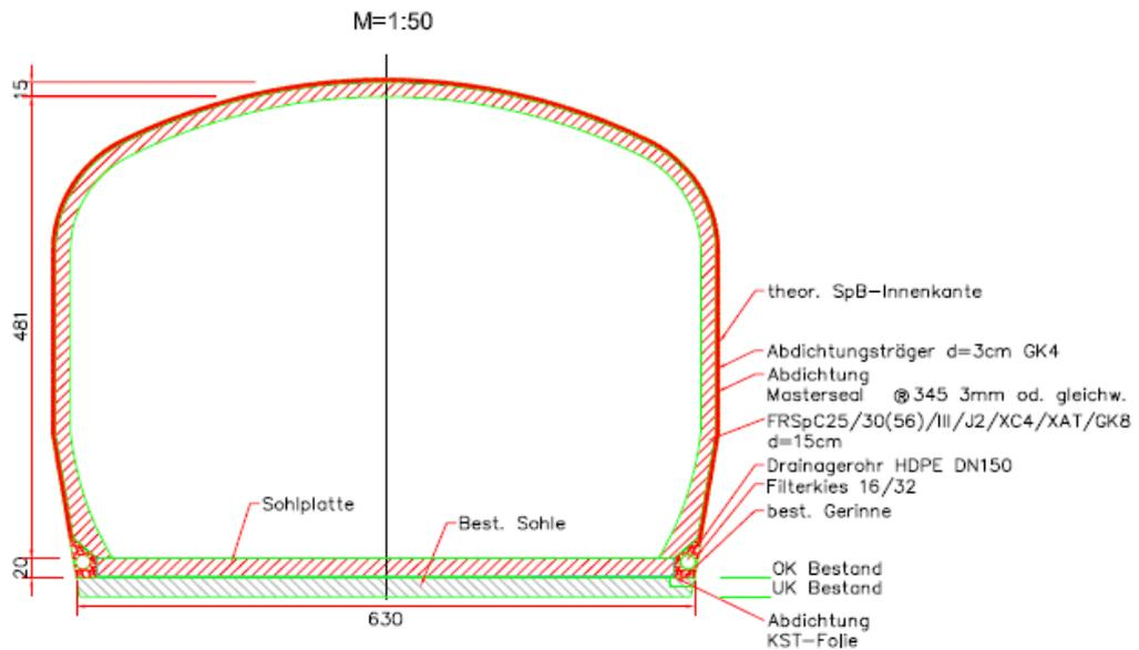
Figure 1: Typical cross section and proposed refurbishment measures [iC]
