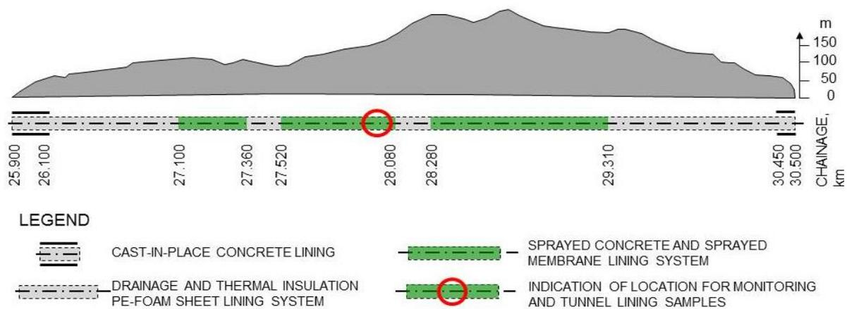
Figure 10: Longitudinal section of the Gevingås rail tunnel, total length 4100 m, showing the different constructed lining types [6]
