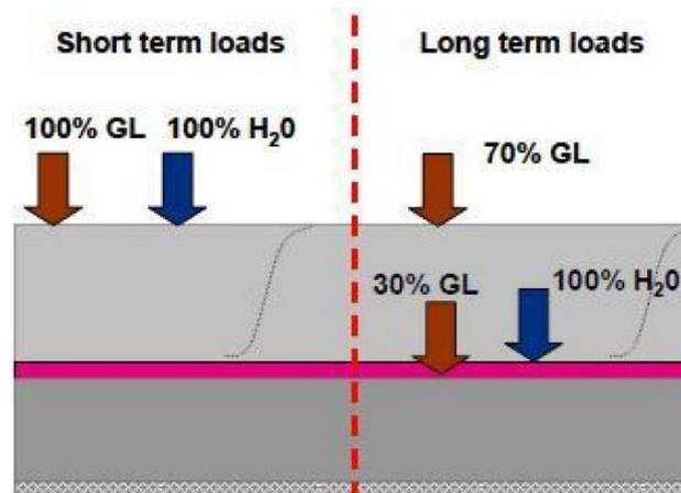
Figure 14: Load sharing between primary and secondary SCL linings [10]
