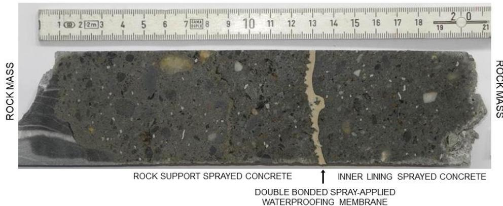
Figure 12: Drill core sample from the complete final waterproof lining [8], drill location shown in Figure 11 right (lining structure detail)
