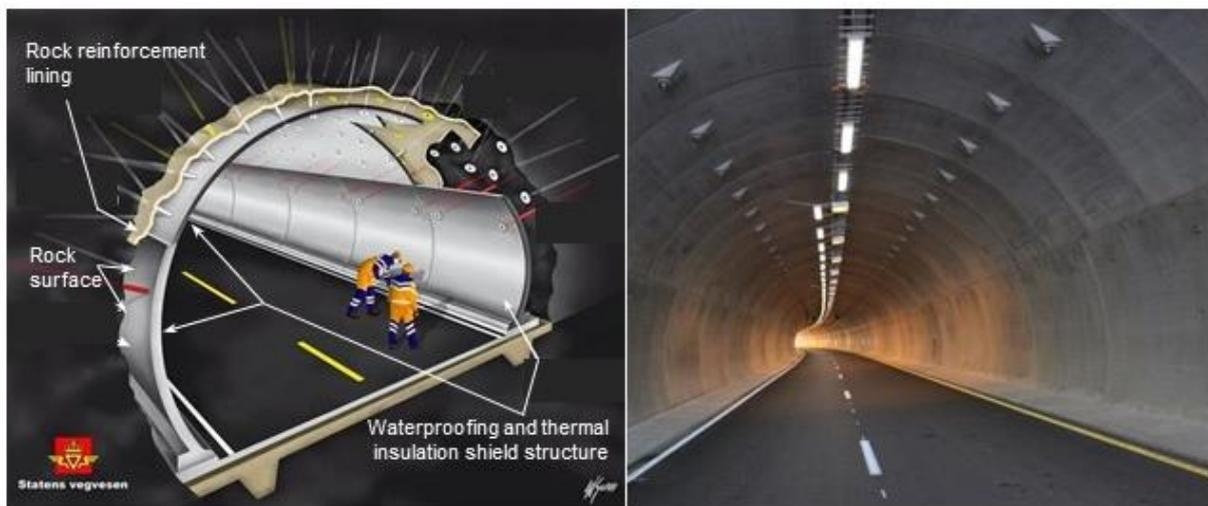
Figure 2: Modern road tunnel design in Norway. Left: illustration of the lining systems rock support and final inner linings. Right: Photo of the interior with final inner lining, the version based on precast segments, for water and frost protection [4].
